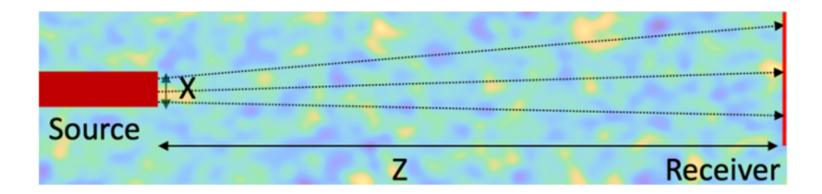
Wave-beam propagating in turbulent atmosphere
