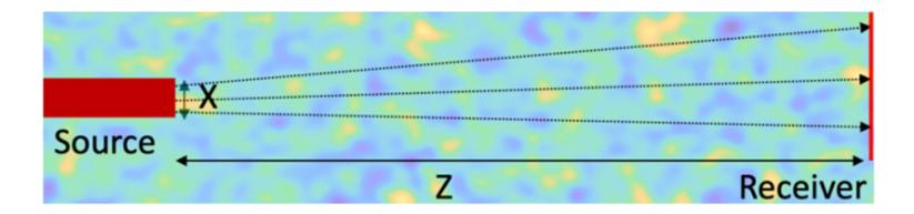
Wave-beam propagating in turbulent atmosphere
