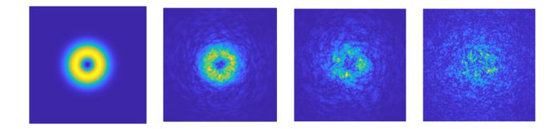
Receiver reading as turbulence strength (or z) increases.
