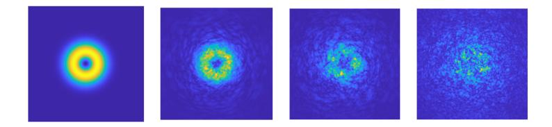
Receiver reading as turbulence strength increases.
